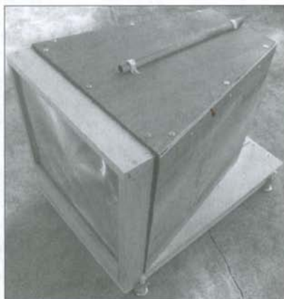
Figure 7: Side view of the PMT 550mm FL box with sighting tube
