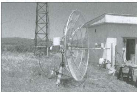
E77DX 9cm - opposite of dish TRV and SSPA connected by hard line to the feed
