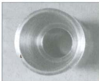
Figure 18 - 1.7\lambda diameter optimum dual-mode horn for 47 GHz
